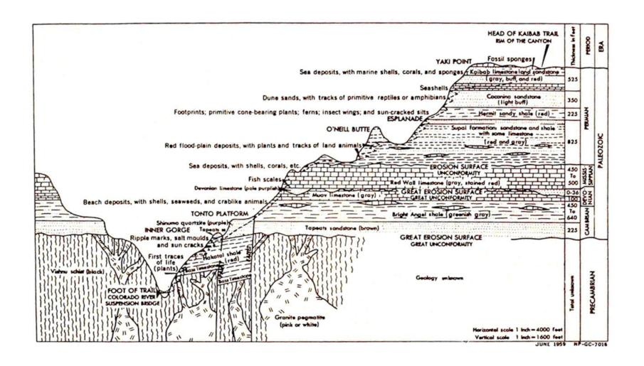
Fig. 26. Vertical section through the sedimentary layers seen on the sides of the Grand Canyon (also of the non-sedimentary layers at the bottom of the Canyon). Note the position of the Redwall Limestone Formation, and of the weathered erosion surfaces which appear just above and beneath it. See text for explanation of these erosion surfaces, and of some of the contrasting layers in the Formation. From "Kaibab Trail Trip Guide Leaflet," U. S. Department of the Interior, 1963.
